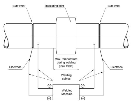
Note: Maximum temperature during welding – see below table (on the drawing exemplary shown  $80[^{\circ}C]$  as for Epoxy coating)
