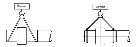
A particular care must be taken not to damage the external or internal coating. If so happens a repair procedure supplied or approved by the manufacturer must be used (*after submitting the demand*).
