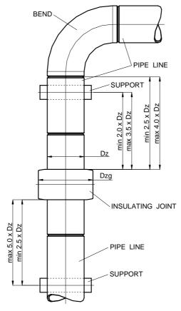
Final distance parameters stipulates design office on the basis of calculations related to type of pipeline (*above or below ground*), established external loads, the supports spacing, the soil type, assumed shape of pipeline, etc.
