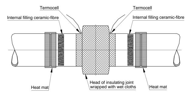
In case of insulating joint's damage due to heat generated during welding process or PWHT, insulating joint shall be replaced by New one. Damaged insulating joint, due to overheating, can be identified in two ways:
